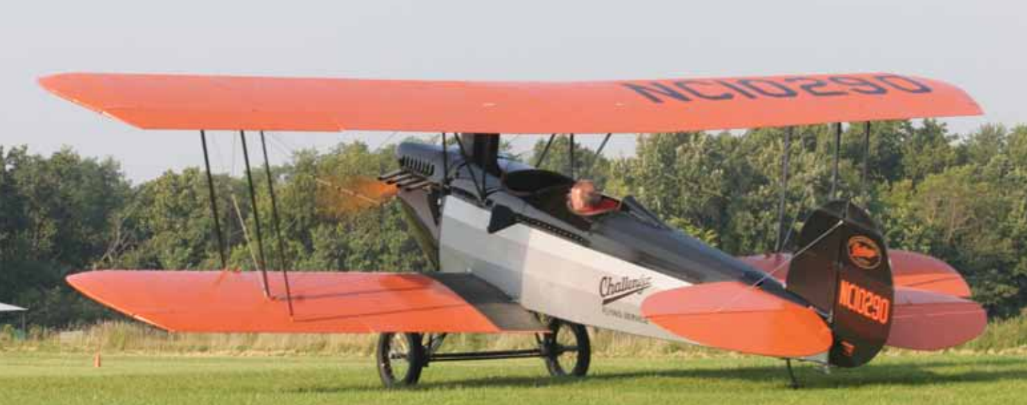
The OX-5-powered KR-31 has four ailerons, which are activated by push-pull tubes.
