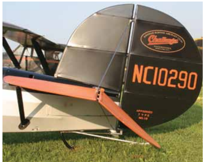
There's no mistaking the rounded tail of the KR-31. D.J. Short modified the tailskid to make it steerable.
