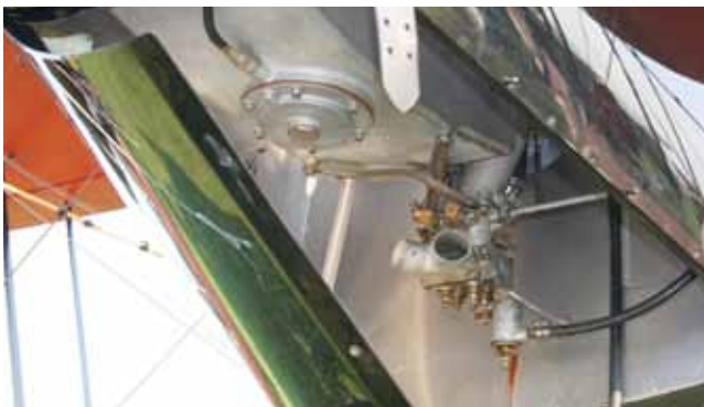
The lower cowling is opened during preflight to permit access to the fuel drains.
