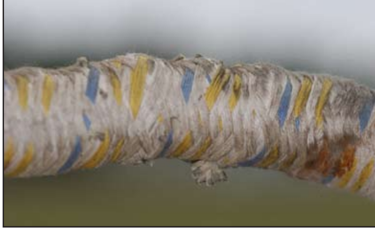
This cord shows obvious signs of damage to the outer covering and to the rubber strands inside. The bumps and breaks in the covering indicate many broken strands of rubber inside the shock cord. This cord must be replaced.
