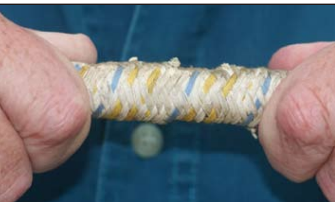
Most normal humans would not be able to pull on a 3/4-inch shock cord and be able to stretch it, but this cord had deteriorated to such an extent that it was possible for me to do so!
