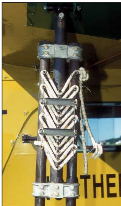
Some aircraft use multiple shock cords. This is the upper end of the landing gear of a Fokker Super Universal. A similar herringbone arrangement was used on the Ryan NYP, Spirit of St. Louis.
