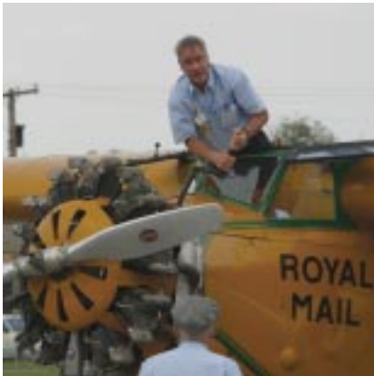
Clark Seaborn got a workout at each stop, hand cranking the inertia starter on the Pratt & Whitney mounted on the nose of the Fokker Super Universal.
