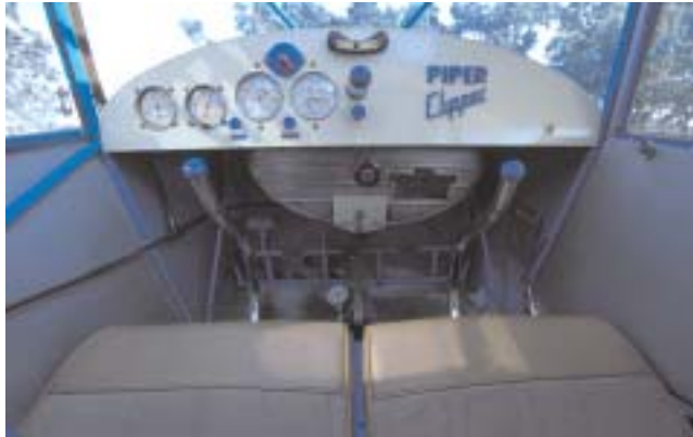
The six instruments required for basic VFR flight (the fuel gauge is in the middle of the tank) plus a slip/skid indicator are all Eric installed in his non-electrical Clipper. To raise and lower the landing gear mounted on the amphibious Murphy floats, a manual hydraulic pump, bolted between the front seats, is used.
